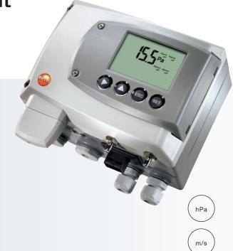
The differential pressure transmitter testo 6351 was developed specially for monitoring differential pressure in the measuring range from 50 Pa to 2000 hPa. For this reason, it is suitable for monitoring cleanrooms as well as for demanding VAC monitoring. In addition to this, the flow velocity or the volume flow can be calculated from the measurement of the differential pressure in a Pitot tube.
